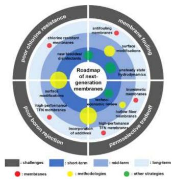
**Fig. 2.** Technology roadmap of the SWRO membrane fabrication, showing different short- and long-term strategies. The size of the circle represents the impacts they are likely to make towards next-generation SWRO membranes.
